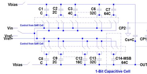
Fig. 4 Unit Split-Capacitor DAC
