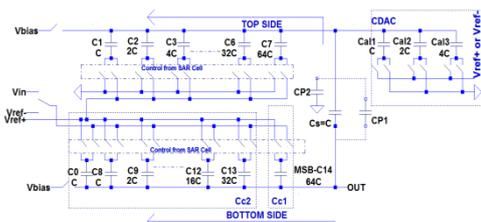
Fig. 7 Unit Split-Capacitor DAC with mismatch calibration
