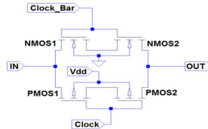
Fig. 3 Stacked Transistor TG as a switch
