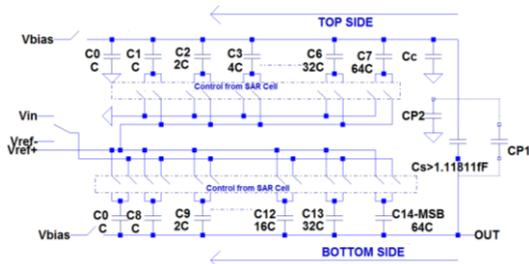
Fig. 5 Split-Capacitor DAC with mismatch calibration
