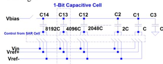
Fig. 1 Capacitive Charge scaling DAC
